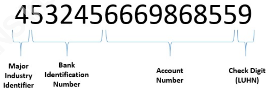
Figure 3 - Card number structure for a Visa card (from Moldes (2014b))
