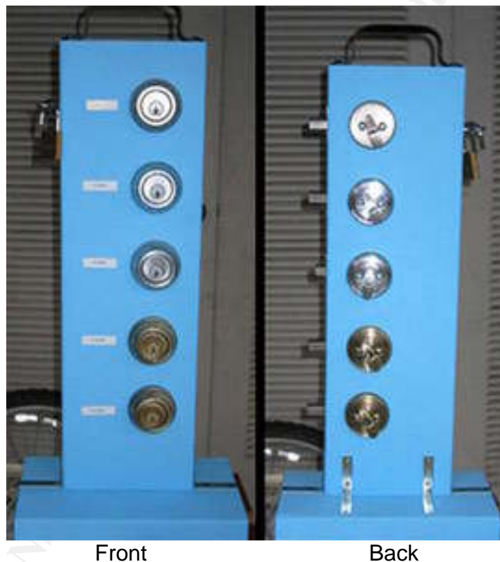
Figure 12. Picking practice board with deadbolt locks 40
