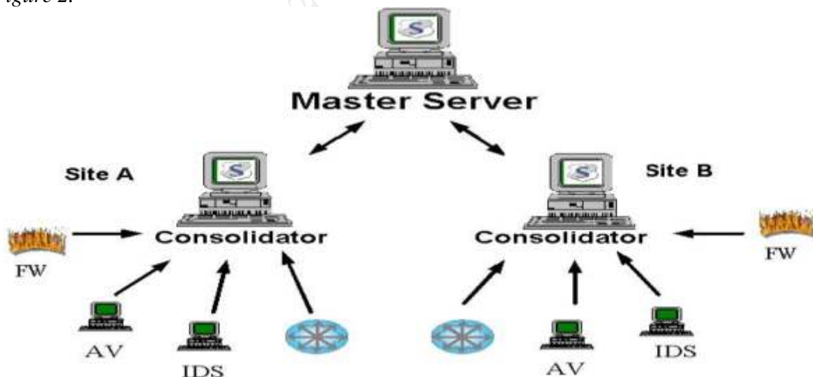
Figure 2: The SSM architecture lends it self to be very scalable. This figure shows three geographically separated sites. The site with the MS and the two sites with CS's. Information is filtered and correlated at site A and site B separately and then sent up to the MS station where it is filtered and correlated again and alarms and alerts are generated. This way we limit the traffic and load for the MS station.
