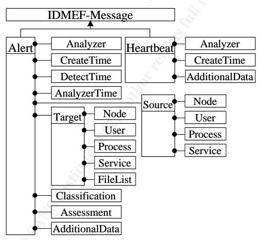
It is important to note that the data model does not specify how an alert should be classified or identified. For example, a port-scan might be identified by one analyzer as a single attack against multiple targets while another analyzer might identify it as multiple attacks from a single source. However, once an analyzer has determined the type of alert it plans to send, the data model dictates how that alert should be formatted.
