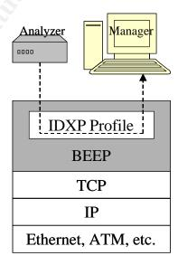
BEEP framework is used as the basis to derive an Intrusion Detection Exchange Protocol (IDXP). It allows authentication and confidentiality through the use of 'profiles.' So a profile is
