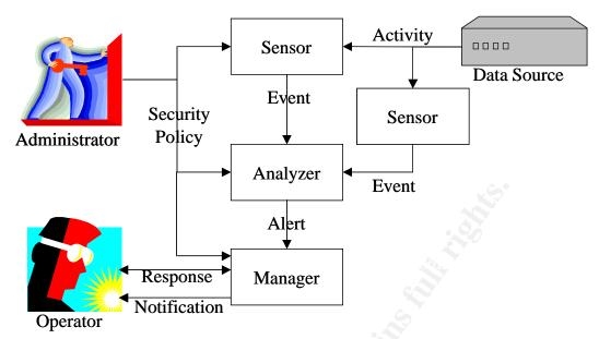
The diagram above illustrates the terms described below and their relationships. Not every IDS will have all of these separate components exactly as shown. Some IDSs will combine these components into a single module; some will have multiple instances of these modules.
