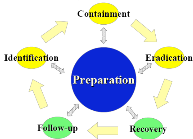
Figure 3--SANS 6-step incident handling methodology
