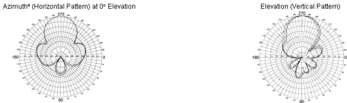
Fig 2. A directional antenna.
