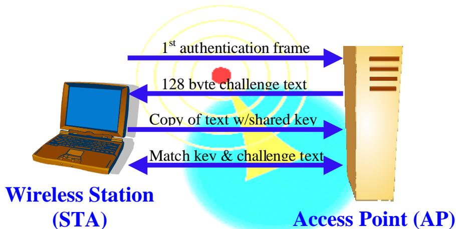
Figure 2: Graphical illustration of the shared key authentication process.
