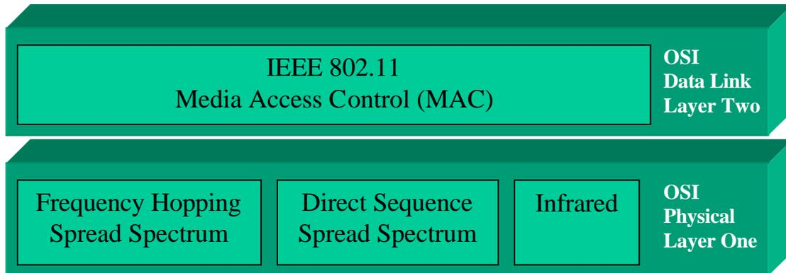
Figure 1: The OSI model according to IEEE 802.11 protocol.
