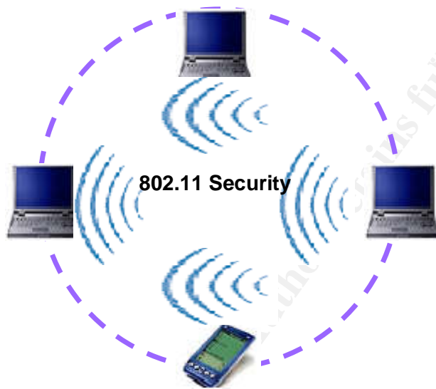
Figure 1 - 802.11 WLAN Implementation In Ad Hoc Topology
